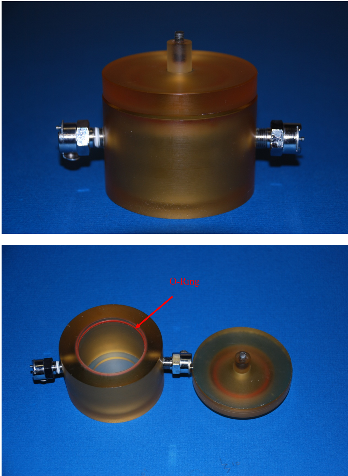
Figure 3-3: Bioreactor chamber with lid closed (up) and open (down).
